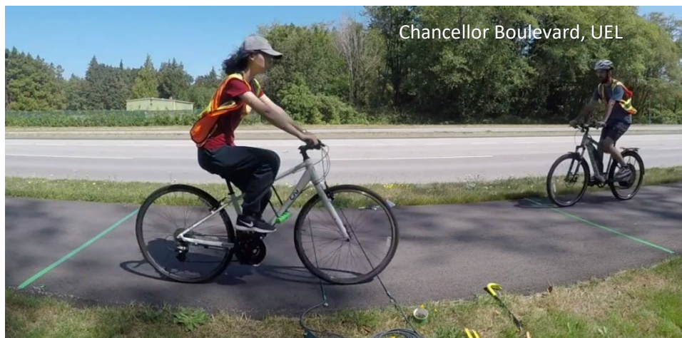
Figure 41. The set-up of testing the accuracy of pneumatic tube's speed measurements against ground truth (speed from video recordings)
