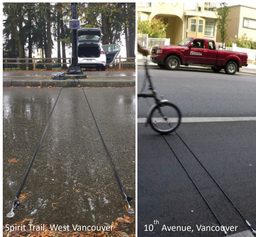
Figure 7. Classified count and speed data collection instrument (pneumatic tubes and a camera)
